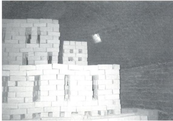
Figure6: Pillar setting (packing) inside an igloo kiln.
